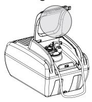
1) Slightly lift up the lid so you can insert the shackle through the hole in the lock tab. This will allow room to get the lock shackle slid into position.
