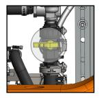
**3)** Power on sprayer pump using the switch on wire harness. If there is liquid in the tank and the valve in step 2 is in the open position, the pump should prime automatically.
