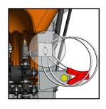
**4)** Adjust regulating valve to aquire desired pressure. Start by threading the regulating valve all the way down (clockwise), then back off 3 revolutions (counterclockwise).
