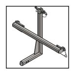
**2)** Take 3/4" x 4-1/4" quick connecting gold pins and insert into two lower mounting points connecting receiver hitch to unit.
