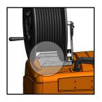
**4)** Connect 1/2" hose reel feed line to hose barb connection on the reel with supplied 1/2" hose clamp.
