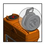
**2)** Secure hose reel frame to tank with provided hardware.
