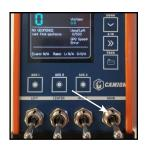
**2)** Press the A/M button to activate 'Manual' mode allowing you to test valves are operating.
