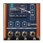
3) Turn 'Left', 'Center', and 'Right' toggle switches on to verify the unit is connected and then turn back off to close the valves. You should be able to hear the valves opening and closing.
