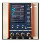
2) Press and hold settings button on the top right corner of the screen for a couple seconds or until it activates a long beep.
