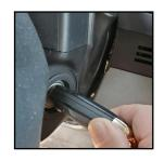
2) To power up the receiver box at the back of unit, plug the RV socket into the 7 pin plug on back of truck.
